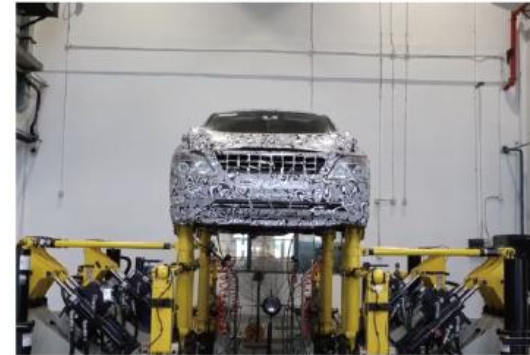
Vehicle Axle Coupling Road Simulation Test
