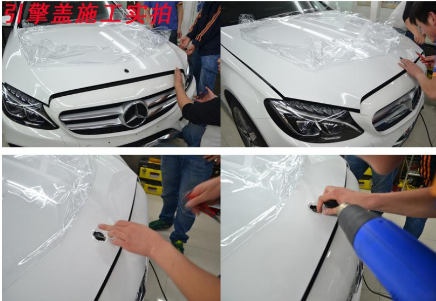
Photos of engine hood film application construction
