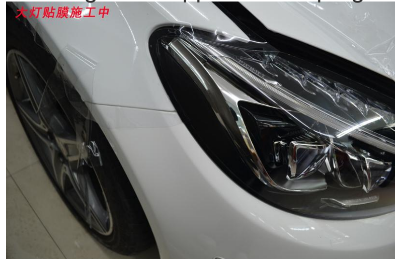
Headlight film application in progress.
