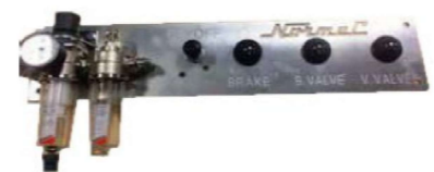
10.52.49 (1) Control panel WITH FRL group, push-pull and pneumatic light
