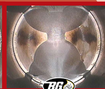
AFTER: Piston crown after BG Gasoline/Air Induction Service.
