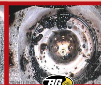
AFTER: Cleaned GDI Injector tip
