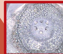
BEFORE: Accumulated hard-to-remove deposits on the GDI Injector tip
