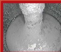
BEFORE: GDI Intake valve with heavy buildup of carbon deposits.
