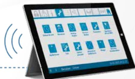
**Smart.** It is possible to operate the ISU Mobile with another control unit (e.g. from another workstation or outside the room to be decontaminated). All operating states of the system, all actual values of the sensors, the process lines, all alarms, and the current cycle data are provided via the LAN interface. The operator can select and start a cycle externally via the LAN interface.
