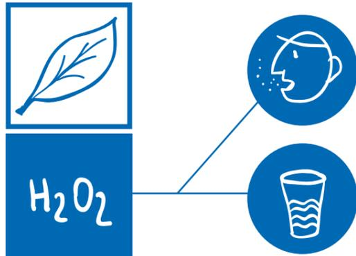
The decomposition of H<sub>2</sub>O<sub>2</sub> does not produce toxic residues (splitting into water and oxygen)
