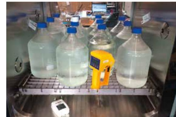
Drying phase of the condensate before H<sub>2</sub>O<sub>2</sub> decontamination
