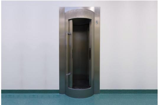
Carousel passbox is designed as a self-supporting independent device of sandwich construction - surface material stainless steel sheet AISI 304 - surface polish 320, filling mineral wool + lead insert Pb, thickness 2 mm.
