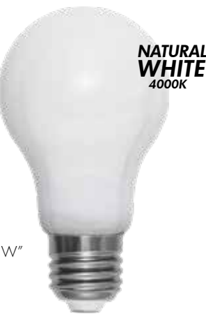
375-51-1 E-NR 8294300 10/100 60mm 107mm 4000K 90Ra 1050lm 10W (≈75W) E27 220-240VAC EC F
