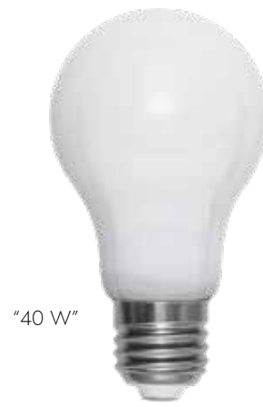
375-32 E-NR 8294313 10/100 60mm 109mm 2700K 90Ra 470lm 5W (≈40W) E27 220-240VAC EC F
