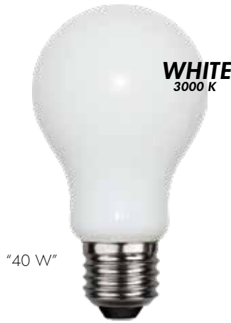
375-31-2 E-NR 8290307 10/100 60mm 108mm 3000K 90Ra 470lm 5W (≈40W) E27 220-240VAC EC F
