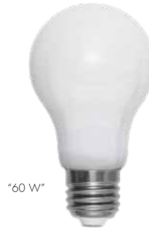
375-42-3 E-NR 8298065 10/100 60mm 107mm 2700K 90Ra 806lm 7.5W (≈60W) E27 220-240VAC EC F
