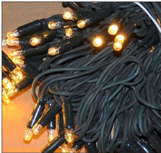
24V LED STRING LIGHT 10MT 98LED, ROUND CAP, DARK GREEN CABLE 0.5MM2,CONNECTABLE. NO POWER CORD.IP44
