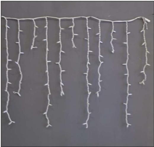
230V ICICLE LIGHT 1.5X1MT 80LED,EACH SEGMENT * 3, RUBBER CABLE 0.5MM2,STRUCTURE 7/10/3/7/10/3/7/10/3/7/10/3,LED DISTANCE 10CM, STRING DISTANCE 12.5CM, CONNECTABLE,NO POWER CORD,IP44
