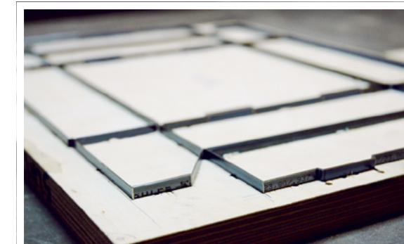
Punching is the cutting of irregular shapes on paper, using a punch.
