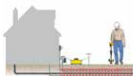
Direct connect to utility lines
