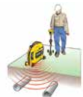
Induce a signal to locate utilities
