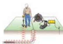
Find plastic pipe with integral line trace
