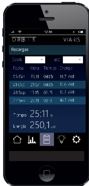
Charge log files between two dates with start time, duration and consumed power.
