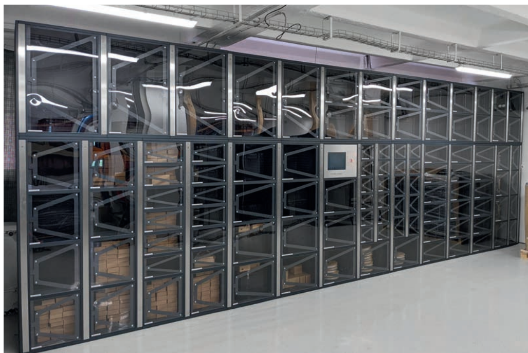
system with special height up to 98,4 inches for management of raw products and produced semi-finished products
