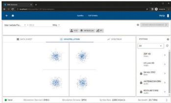
In the measurement you can switch back and forth between the measured values, the constellation diagram and the channel spectrum as in the spectrum view. Thus, the measured values are particularly vivid and can be quickly compared with each other. In the right area, all transmitters or services on the channel are listed. One click takes you to a specific transmitter and its measured values.
