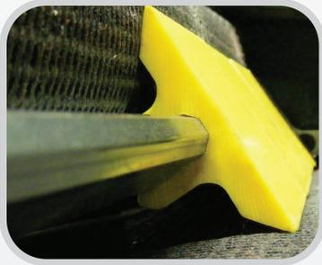
**Snap-fit design:** The 75mm (3") segments are designed to release under pressure if small objects become lodged between belt and segments.
