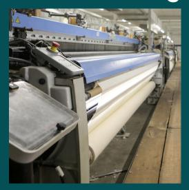
With an in-house capacity of 25,000 meters of napkins & sheets per day, our weaving operations are powered by 36 ITEMA Electronic dobby rapier looms. This ensures efficient production and superior quality for our hospitality linen sector.
