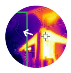
The photo, taken with a thermographic camera, clearly displays the perfect and optimal temperature distribution of the machine and the efficient hot air recovery through the hood, without the operator (highlighted in the green zone) being struck by the heat while remaining in the operating area.
