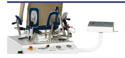
With **6 pneumatic clamps**, to hold each type of jacket or garment, to ensure all possible finishes, also guaranteeing **greater clamping uniformity** during the finishing phase, for better quality both inside the lining and outside the fabric.
