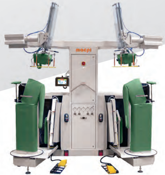
234 Shoulders, sleeves and armhole pressing
