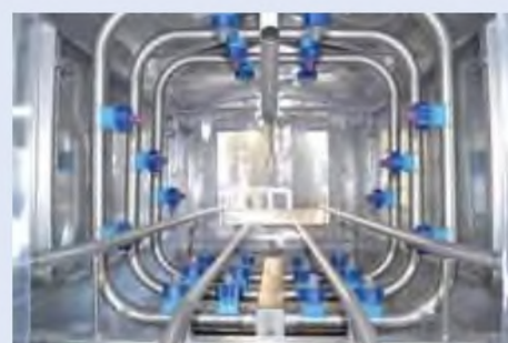
system of nozzles with adjustable direction
