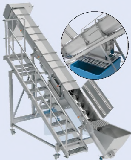
Version with unloading valve
