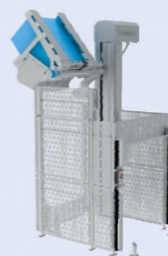
Safety cage with sensors-light curtain type
