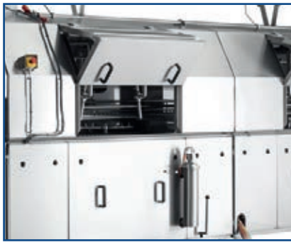
Image 25 2-phase door opening - drying position
