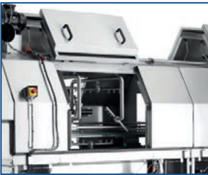
Image 24 2-phase door opening - cleaning position
