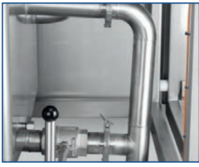
Image 26 Removable piping - optimum accessibility
