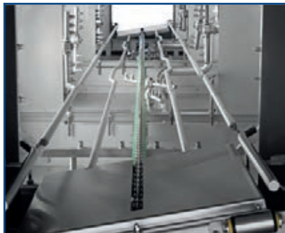
Image 17 Inclined / offset container guidance - no splash shadows
