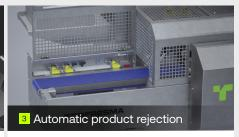
The product rejection mechanism ensures the absence of empty packages and the integrity of the packaged products.
