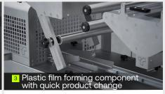
This component allows the film to fit perfectly around the hamburger, ensuring a secure and uniform sealing.
