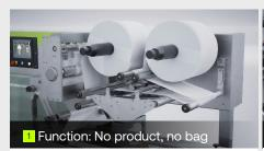
Identifies when there is no product feeding, pausing the process and automatically restarting when a product is detected.
