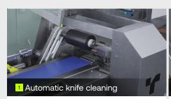
The automatic knife cleaning ensures hygiene and efficiency, preventing contamination and maintaining the quality of the packed products.
