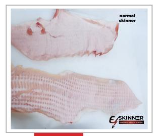
Due to it 's precise cutting technology the **GECO eSkinner** allows to cut razorthin. This cut is approximately 30% thinner than comparable machines. This leads to **less fat on the skin.**
