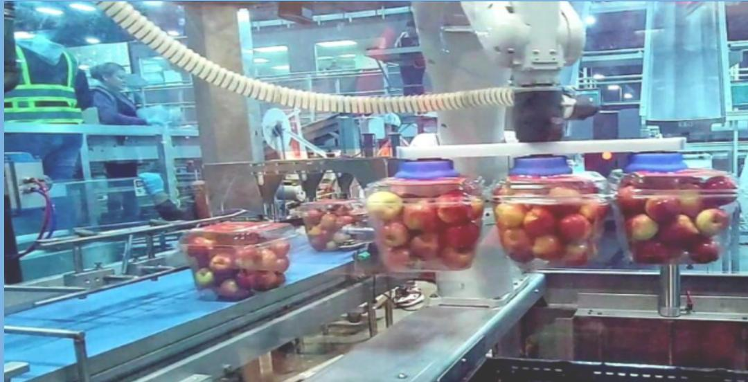
Gripper tool for the Robot case packer solution by Haley Manufacturing inc.
