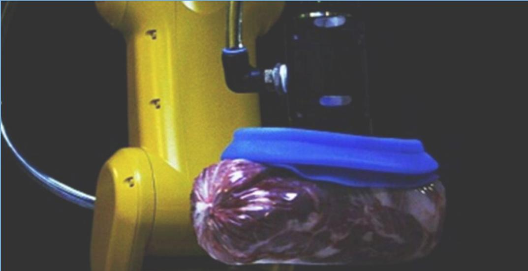
Custom-tailored gripper tool for the multifunctional robotic application. Handling of raw and packed meat pieces.
