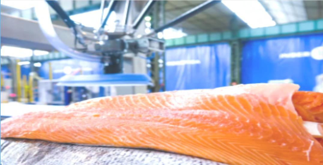
Special end-of-arm tooling for Delta-type robots. A cutting-edge solution for sorting and grouping salmon sides was developed by Inser Robotica.
