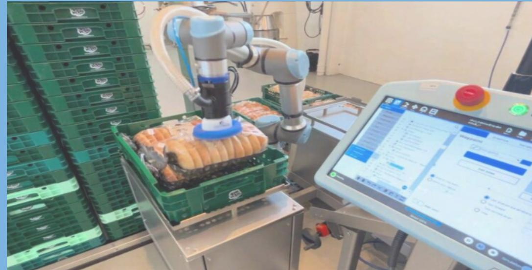
Solution for packing bakery products into crates. Suction cup gripper for handling bags.
