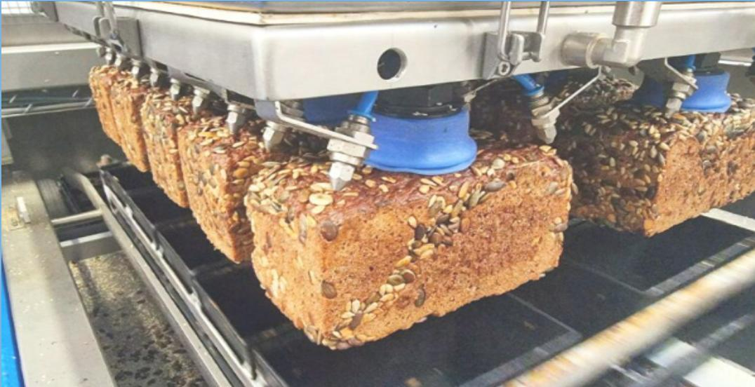
Automatic de-panning of fresh loaves of rye bread with a tailor-made vacuum gripping system.
