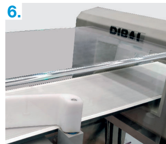
6. Methacrylate tunnel from the detector's arc to the end of the equipment to avoid manipulation of the product after the detection process.
