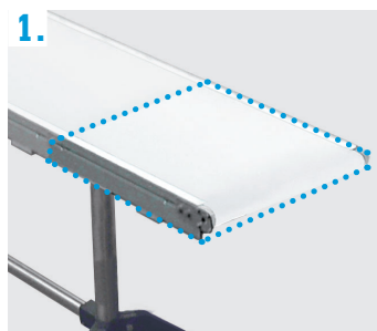
1. An extension of the transport system to place the reject system and the container.
