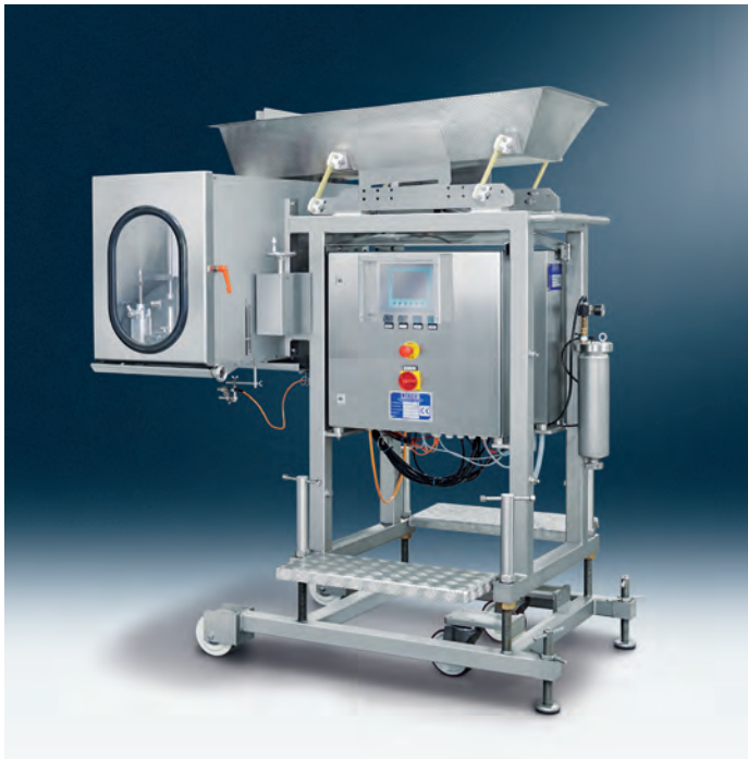
AWF 1, mobile on wheels, lightweight version with 60 l product hopper, controlled through vibration
