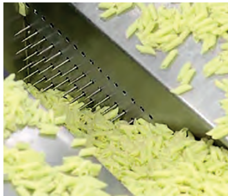
Spaghetti feeder for long fibrous or lumpy products
