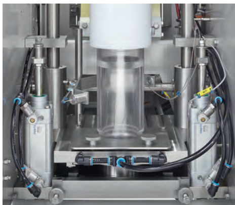
AWF 1, mobile through lift truck, heavy version with 300 l product hopper, controlled through vibration
