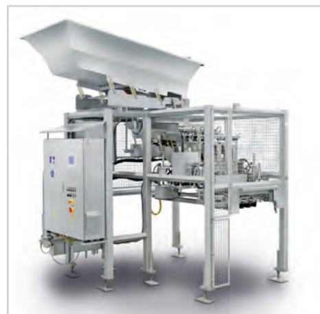
AWF 4 for installation on a machine from a different brand, with 300 l product hopper with product feeding through a lifting and tilting device
