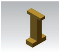
TT = "T" Shaped: a portion of the cleat (usually the upper one) is wider than the rest, so that a cross-section resembles the shape of a capital "T"
