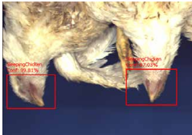
Identifying missing cut after beheading of chicken to ensure all chickens are processed properly and humanely.
