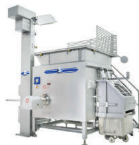
5600 Twin Overlapping Paddle Mixer Mincer with End Discharge and Extended Hopper
