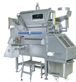
5000 Single Paddle Mixer Mincer with CO 2 Bottom Injection and End Discharge Chute
