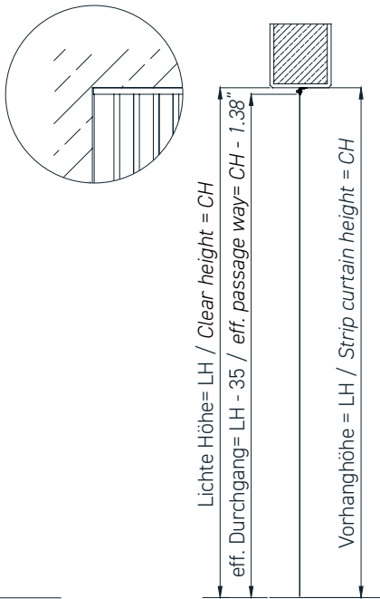
Sturzmontage / Lintel assembly
