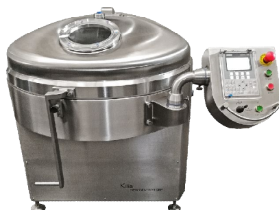
30 ltr Vacuum-Cooking-Cooling Bowl Cutter Manual vacuum lid opening system
