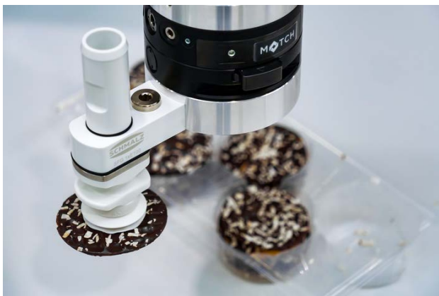
Flow gripper SFG when handling baked goods
