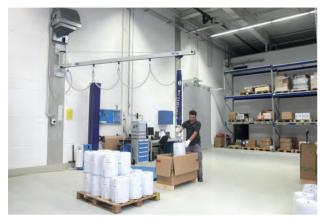
JumboFlex 50 with gripper for jug or bucket handling
