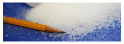
The i<sup>3</sup> MicroClean 2 shaves dry ice into MicroParticles (sugar-sized dry ice particles). Cold Jet's dry ice MicroParticle technology provides a thorough, yet delicate clean for many applications.
