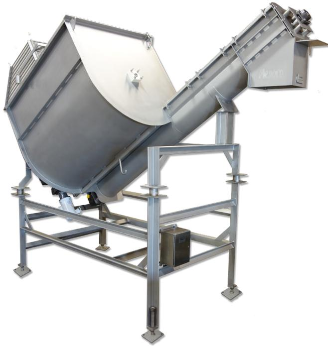
Integral to the Bin Batching System are the Metering Screw Conveyors, designed with a Clean-Sweep hopper. The Clean-Sweep hopper offers a solution that mechanically clears food product between batches on metering or surge loading applications. The ribbon agitator gently and continually pushes product into the feed screw.
