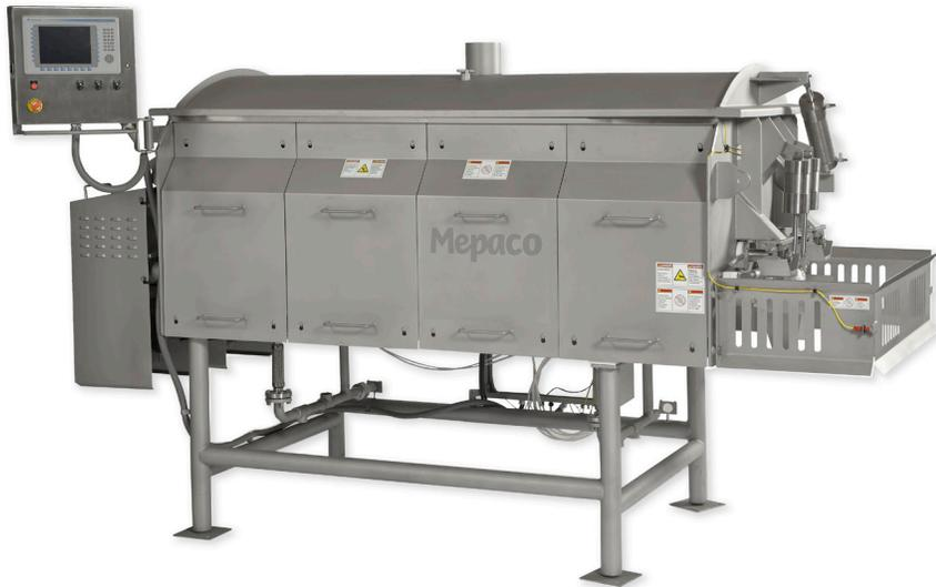
In the system, the food processor required a versatile cooking solution to efficiently blend and cook various soups and sauces, all with different process recipes and controls. The ThermaBlend® was specified for the “Dual Cook System” because of its ability to blend and cook the processor’s viscous products with superior efficiency.
