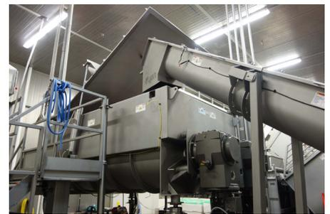
Mepaco's overlapping paddle Mixer-Blenders provide a quick and accurate blend with minimal temperature rise. The Mixer-Blenders in the Pre-Blend System are both equipped with vacuum sampling (image upper right) capability to confirm the actual lean-point for accurate formulation.
