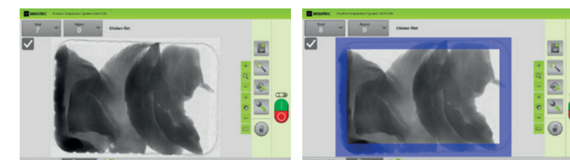
Automatic edge recognition for packaging
