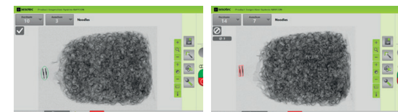
Ignoring metal clips to increase detection sensitivity
