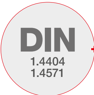
DIN 1.4404 (AISI 316 L), DIN 1.4571 (AISI 316 Ti) or other chemically more resistant stainless steel
