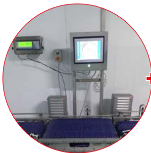
Control stations (I- and C-points) for sorting the material (optional)
