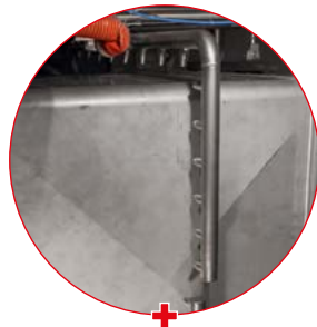
Blow-off nozzles for IBC container exterior drying
