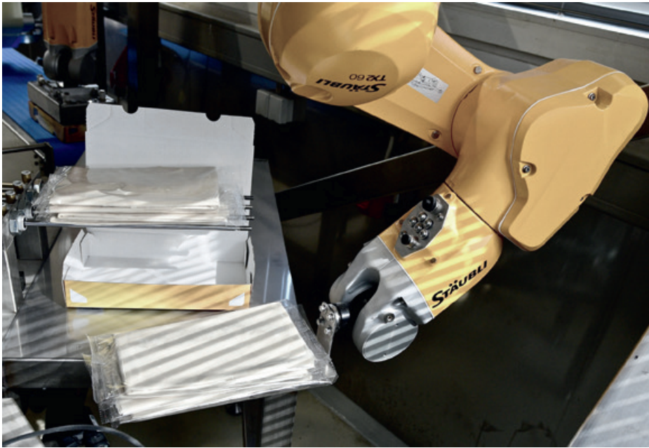
Sisi, a Stäubli TX2-60 robot, picks up four foil-wrapped units at a time and inserts them into the box presented by Franz.
