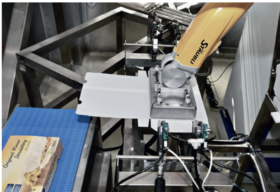
Franz, a TX2-60L, takes a flat-pack box from a stack, guides it along four glue nozzles and presses it into a negative mold. The outer packaging is now ready to be filled.
