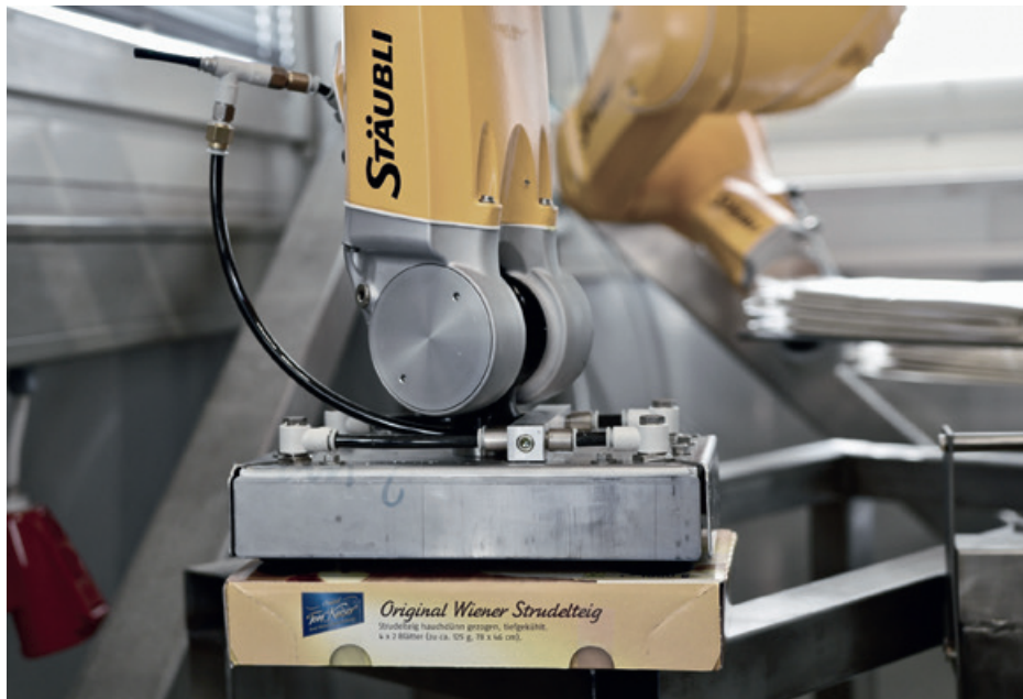
Thanks to the superior safety technology of the Stäubli control system, it was possible to configure the entire packaging cell without a safety barrier.
