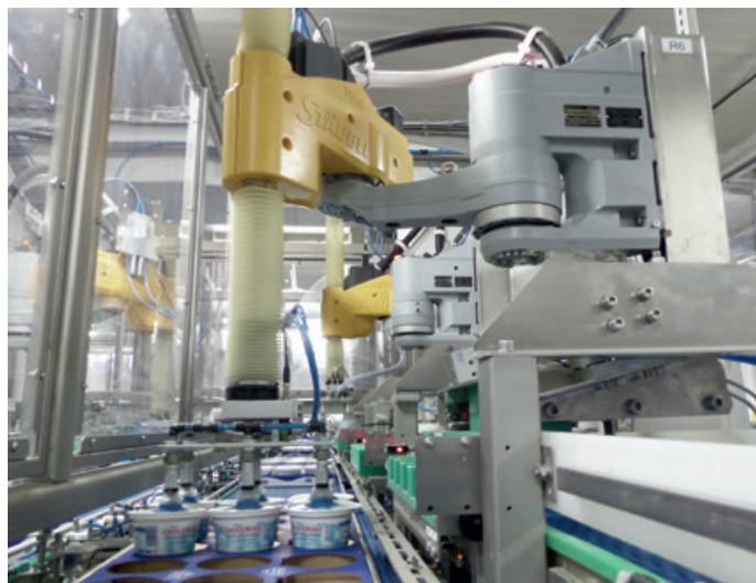
Four TS60 SCARAs pick the tubs off a conveyor belt as they leave production and place them in boxes on a parallel conveyor belt.
