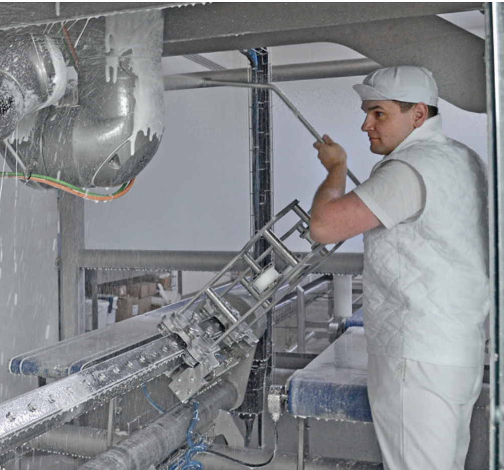
The requirements of cheese dairies are particularly high, given the use of bacteria and other types of microbes. The equipment is cleaned with fat-dissolving, alkaline and milkstone-dissolving acidic agents, and with water heated to 55°C. Image: Plangger organic cheese dairy in the Austrian Tyrol
