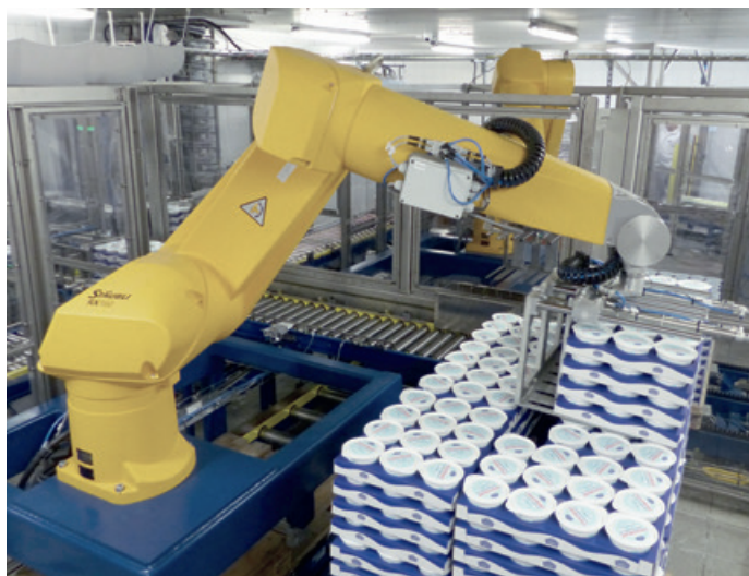
Two six-axis RX160s stack six four-tray layers per pallet, each layer consisting of six cartons. That makes a total of 1 728 tubs per pallet.
