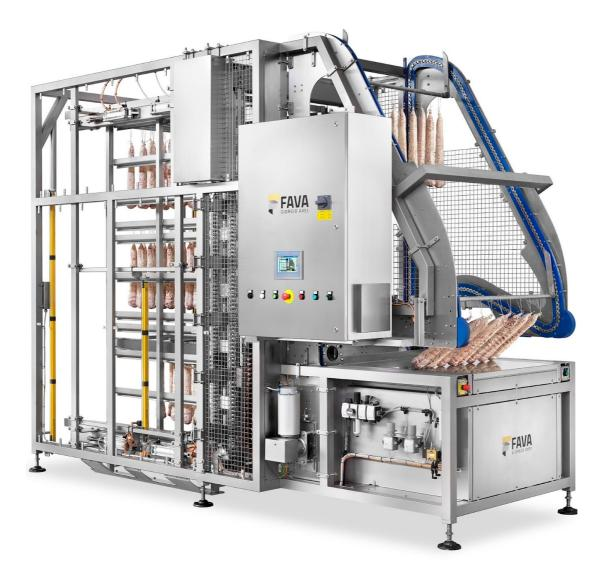
Our CSC series **compact loaders and unloaders**, for racks, frames, trolleys or suspended tray conveyors on which placing poles with hanging products, are the best answer to eliminate tiring, repetitive and risky **operations**, even with a focus on lower throughputs.
