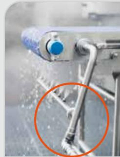
The CIP unit can be mounted on the right or the left side of the conveyor.
