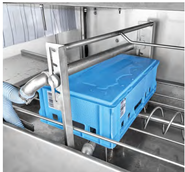
Type DLWA-A 180 Ecoline, detail air knife
