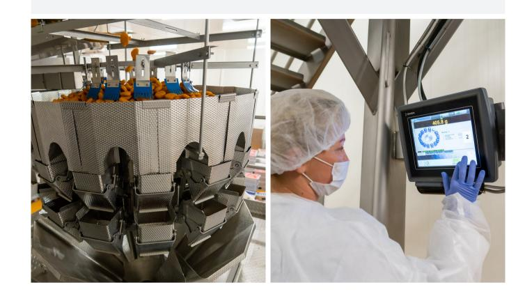
The Ishida CCW-RV-214W-1S-30-WP multihead weigher, a 14-head models with 3 litre hoppers, at Roldrob's plant in Tomaszów Mazowiecki is handling a range of fresh, chilled and frozen products, including breaded items such as chicken nuggets. The weigher has replaced a manual weighing process and, as the company's production manager Sławomir Kołodziejek confirmed, the result has been emphatic.
