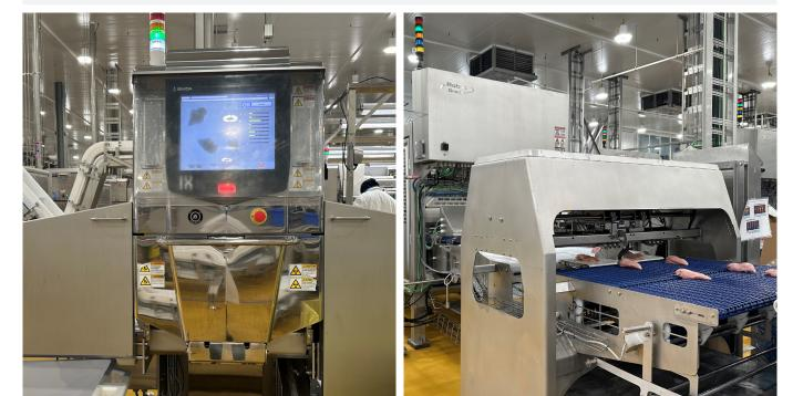
One of the most technologically advanced facilities in the world, the London Poultry Plant features 12 Ishida Flex Grader systems and four Ishida RobotGraders, working in conjunction with four Ishida IX-G2 X-ray inspection systems. The Ishida equipment is able to handle and pack all the cut-up components from the 27,500 birds processed every hour, delivering around 270,000 retail trays each day across the 16 grading and packing lines.
