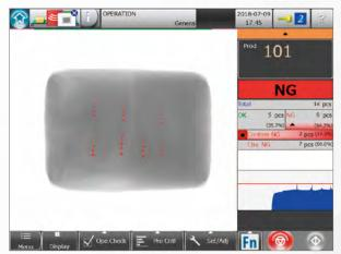
Example: Flour packed in a large bag XR75 software helps operators work more efficiently, displaying reject images on the screen to easily identify contaminants.
