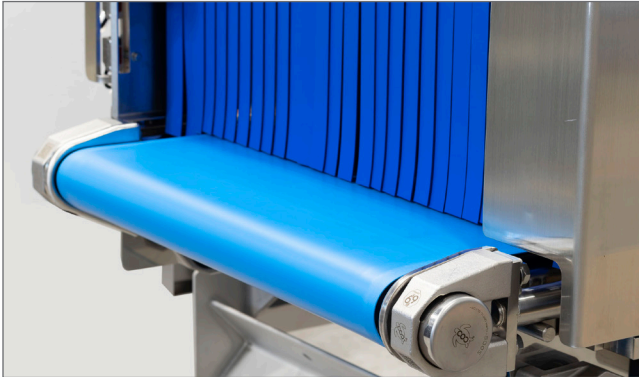
Heavy-duty solid rollers, pillow block bearings, blue sealed belt
