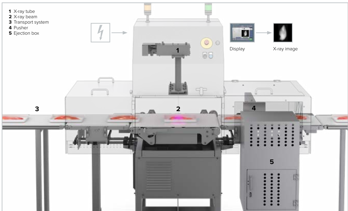
Fig. 2: Design of an X-ray scanner
