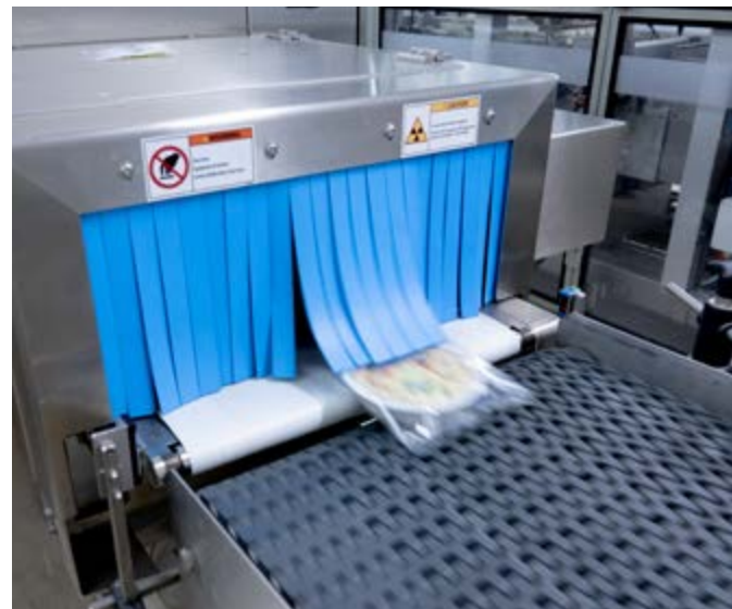
Fig. 1: Frozen quiches are inspected for foreign bodies with an X-ray scanner
