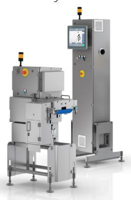
X-ray inspection systems offer a wide range of applications such as foreign body detection, completeness check, filling level check, shape check, position and distribution control, clip examination (closure), mass determination, break and
