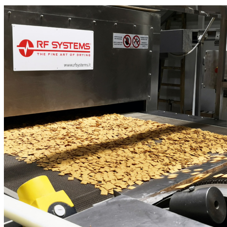
> Drying of crackers 600 Kg/h throughput
