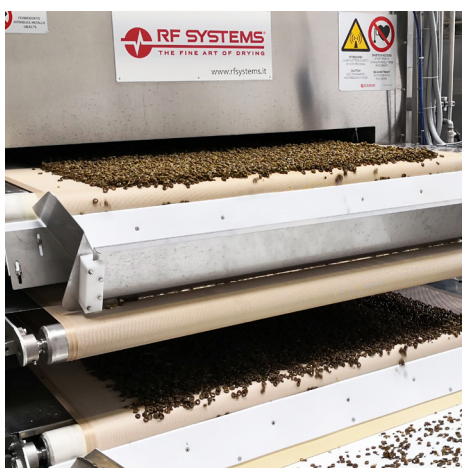
> Drying of candied fruit citrus 1000 Kg/h throughput
