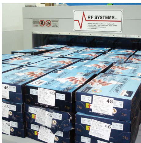
> Defrosting of packaged shrimps 1500 Kg/h throughput
