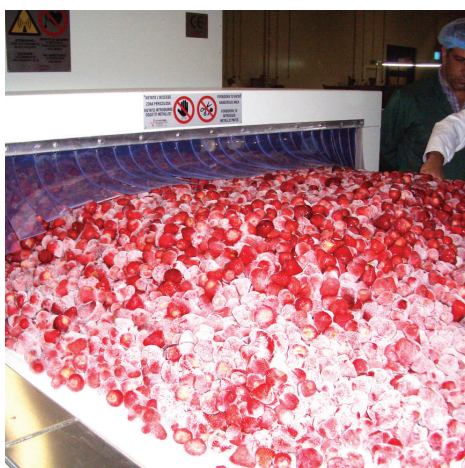
> Defrosting of IQF strawberries 1000 Kg/h throughput
