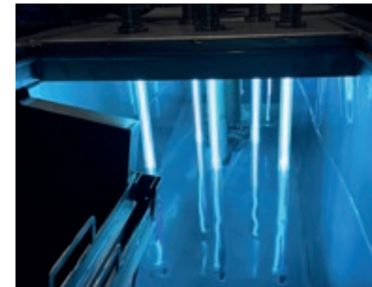
sterilAir® EQ modules integrated in the water tank of a painting line.
