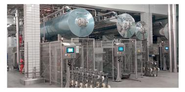
Energy and water management occurs at the autoclave level, but it can also be integrated at the global level of the factory. The hot and cold water recovery system recycles water for subsequent
