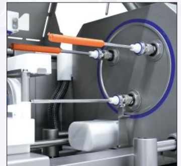
Voider system defines the portion length
