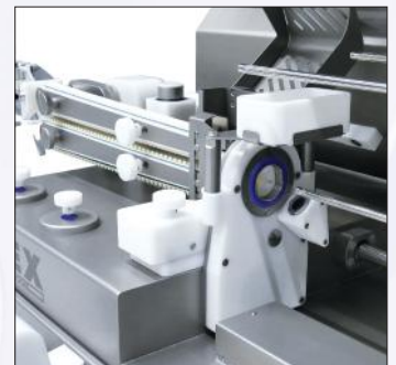
Voider system defines the portion length
